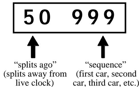
The "splits ago" and "sequence" numbers will be continuously shown while **Print** is actuated. The numbers are also briefly shown whenever the **Recall** toggle switch is actuated. If you hold the **Recall** switch in place, the 650 cycles through the datalog memory, incrementing and decrementing the "splits ago" and "sequence" numbers appropriately.
