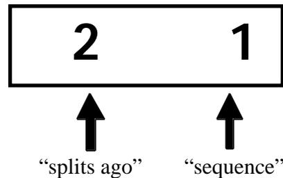
The “splits ago” count has increased to “2”. The data was collected “two splits ago”. The sequence number remains at “1” because the split data being viewed is still the log entry sequence number for the first car.
