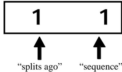
The “splits ago” value is now “1” because that is how far the data is removed from the live clock. The sequence is also “1” because the data is for the first car.
